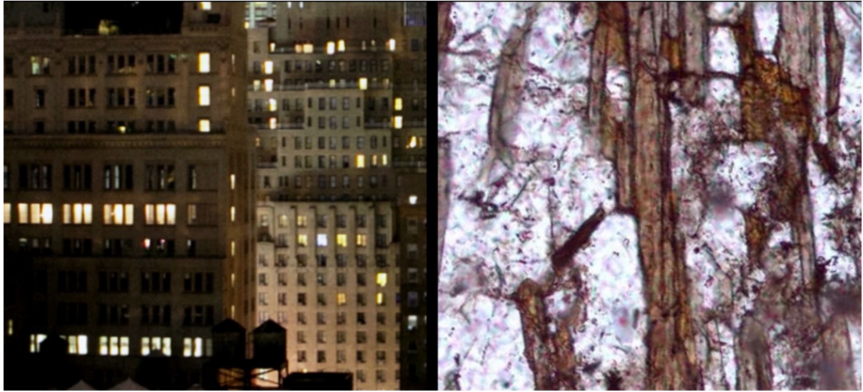
MMM 01 Biotite (Iron Magnesium rich) blades and intergranular Quartz
