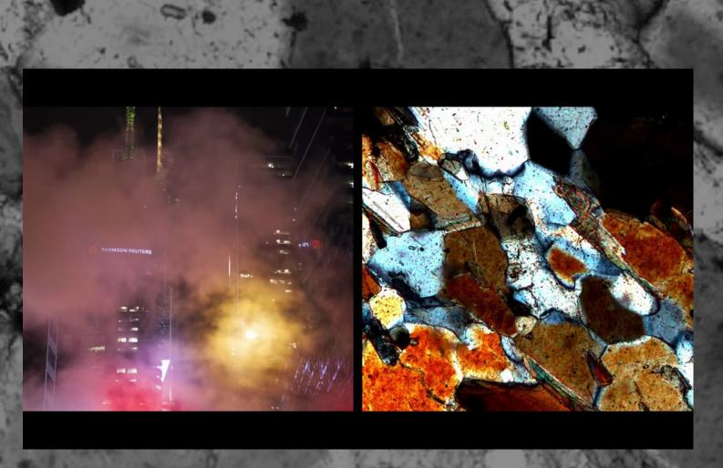
Mosaic of dirty Quartz, this happens when the rocks are not grinded to a 5 micron thickness.
